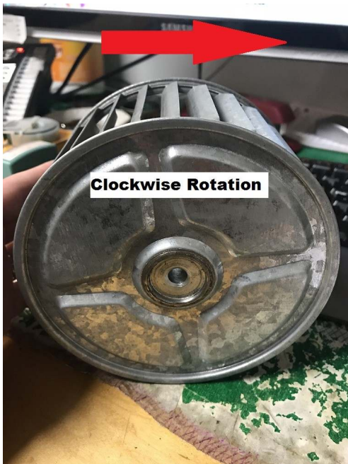
Single Inlet Blower Wheel - Clockwise Rotation - viewed from the Back Plate / Closed End
