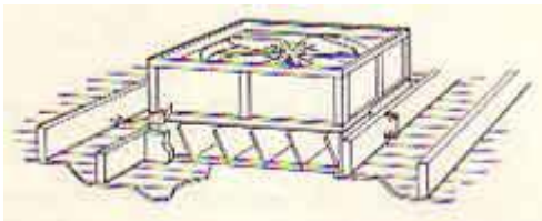
Detail of a vertical discharge fan installation
