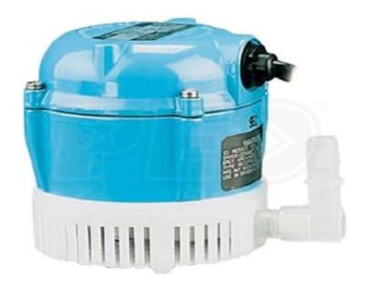
Specs: Horsepower- 1/200 Voltage- 115V Flow at 1 FT Head- 170 GPH Shutoff Head (ft)- 7" Cord Length- 3' Discharge- 1/4" MNPT
